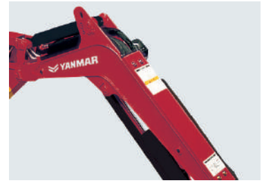
The boom hose and cylinder are covered for protection.
