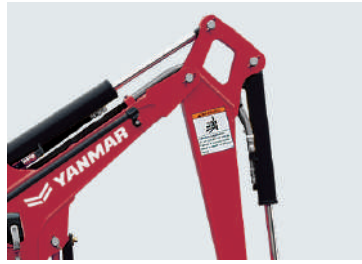
Bucket cylinder hose designed inside the arm.
